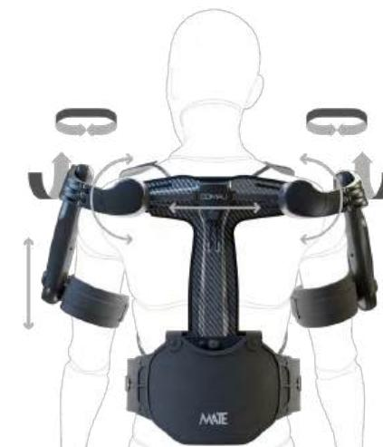
Thanks to a chain of passive degrees of freedom, the human shoulder flexion-extension axis is aligned with that of the MATE-XT GO.
