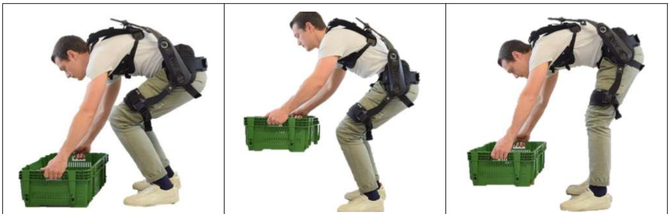
Fig. 2.1 - Example of movements assisted by MATE-XB
