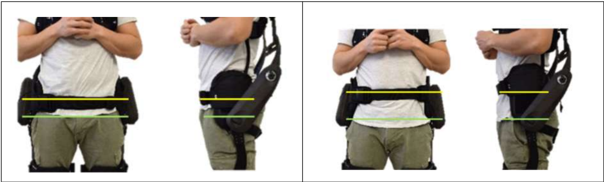
Fig. 4.1 - Pelvic belt height
