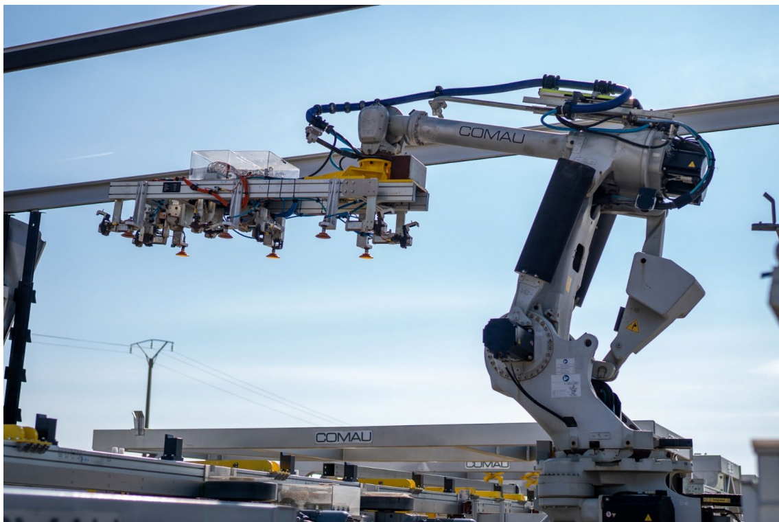
Figure 5.10.: Engineered for outdoor automation, the Hyperflex mobile factory operates directly in the field to optimize the logistics flow. Image credit: Daniel Mora
