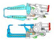
The transformation from X to C (and vice versa) is fast and easy. Simply change a single module, pulley and belt.
