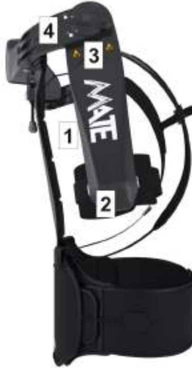
Fig. 3.4 - Torque Generator Box: overview
