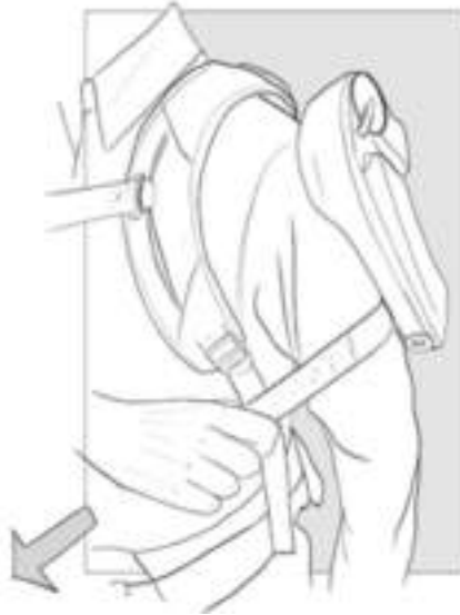
Fig. 5.7 - Torque Generator Box activation procedure
