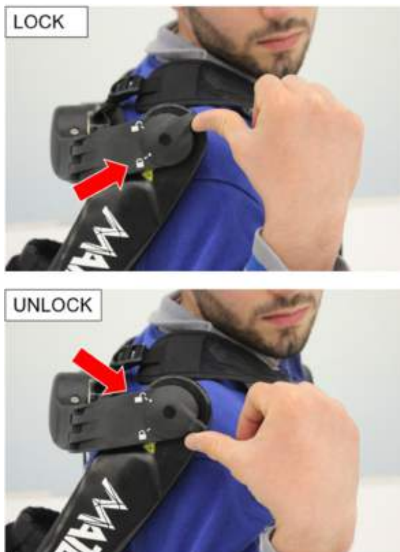
Fig. 3.6 - Torque Generator Box (TGB): locking mechanism
