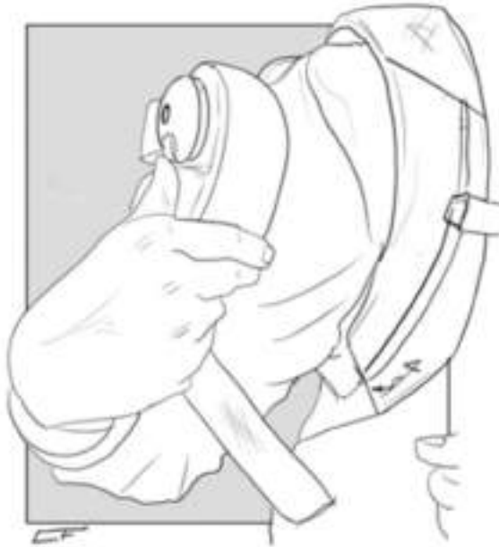
Fig. 5.15 - Locking the TGB locking mechanism
