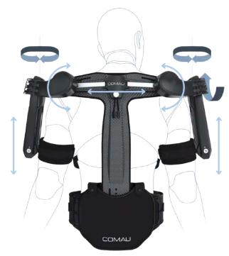
Thanks to a chain of passive degrees of freedom, the flexion-extension rotation axis of the human shoulder is aligned with that of MATE-XT
