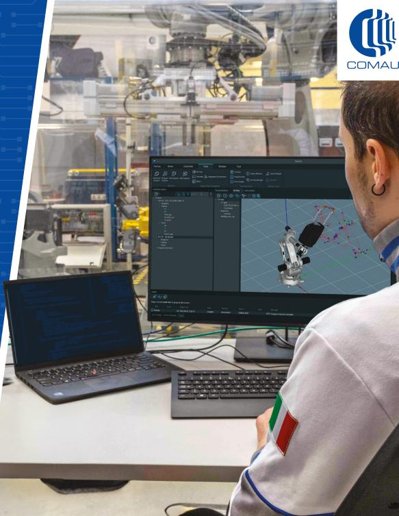
**Comau Open Controller** is a Comau product that implements a fast connection between an external PC and Comau robots, granting the possibility to use additional and custom control algorithms and novel trajectory generation methods.
