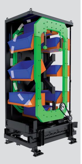
The automatic rotation system to position the shelves is powered by a motor located inside M.I.O. automatically connected (plug and play) to the frame.
