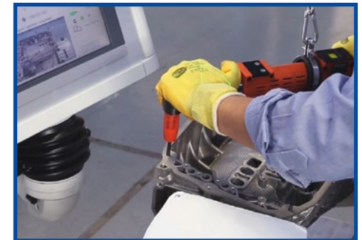
The technological process is enabled only when hands are in a correct position
